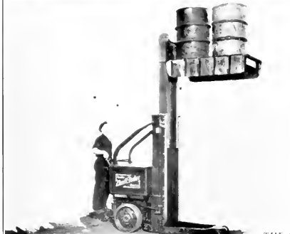
The Elwell-Parker new telescoping, tying truck, normally and extended.
